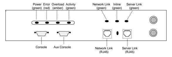
Figure 2-3: Front Panel Connectors and LEDs
